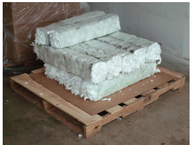
Equivalent amount of scrap compacted into dense logs
