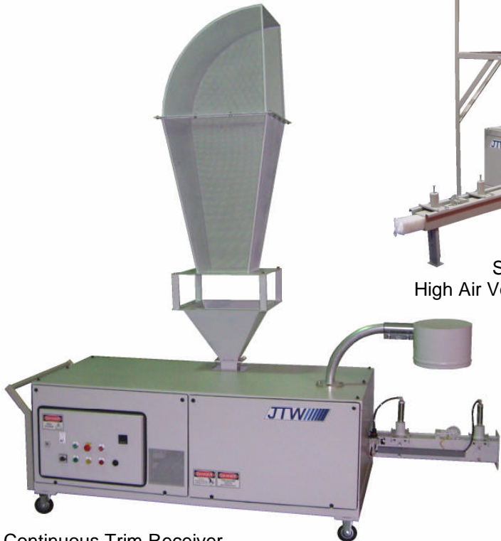
Continuous Trim Receiver shown directly mounted to Poly Compactor
